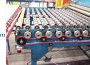
accommodating any size conveyor, has a smooth/flexible top surface that conforms to machine variations and more than adequate strength for transmitting the needed power.
